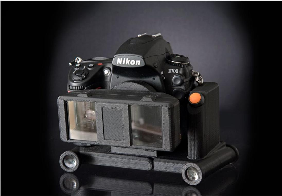
Figure 8. MAVIS Stereoscopic camera. An adapted stereo lens for the Nikon D700.
