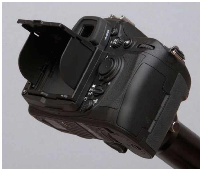
Figure 3. Delkin Devices DVD300-P Hood attached to Nikon D300 body. The hood enhances the use of Live View mode as it helps prevent extraneous light from reflecting on the LCD panel.
