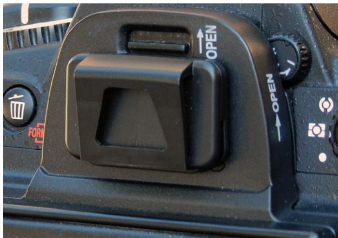
Figure 5. Nikon DK-5 eyepiece cap attached to Nikon D300. Covering the eyepiece prevents any light from hitting the camera's CCD when shooting in Live View so exposure metering is not compromised.
