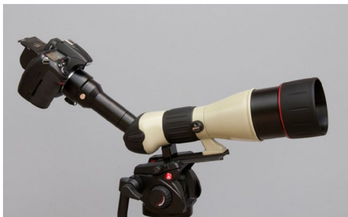
Figure 2. Nikon Fieldscope ED82-A, with Digital SLR Camera Attachment FSA-L1, and Nikon D300 DSLR camera body, connected to Manfrotto 501PLONG Rapid Connect Plate, mounted on a Manfrotto 501HDV head, and Bogen/Manfrotto 3221W aluminum tripod.
