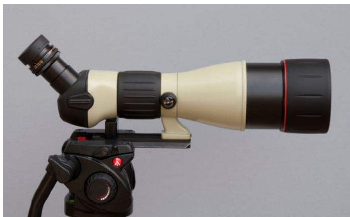
Figure 1. Nikon Fieldscope ED82-A scope with 82mm objective, 1000mm focal length, all-metal, f/13 aperture lens, with sliding sunshade, 45° angled zoom MCII 25-75x removable (threaded) eyepiece. Custom acrylic & dense foam lens support was fabricated to help reduce vibrations.
