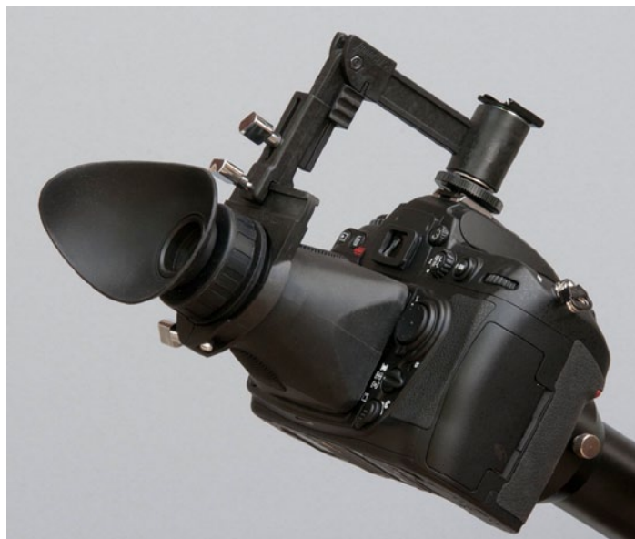
Figure 4. Hoodman Hoodcrane and Lupe attached to Nikon D300. Similar in appearance to a video camera's eyepiece, the 8x lupe provides an excellent magnified view of the LCD's surface, in addition to preventing any light from reflecting on the LCD panel. Unit can also be retracted up from the LCD panel when not in use, or for cleaning the LCD panel.
