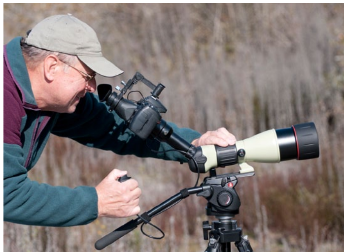
Figure 6. Author focusing scope and preparing to press electronic shutter release (Nikon MC30 Remote Cable). Developing a strict shooting protocol: "pan/tilt....focus....shoot" is necessary in becoming a successful digiscoper. (Photo by Thomas S. Merrill.)
