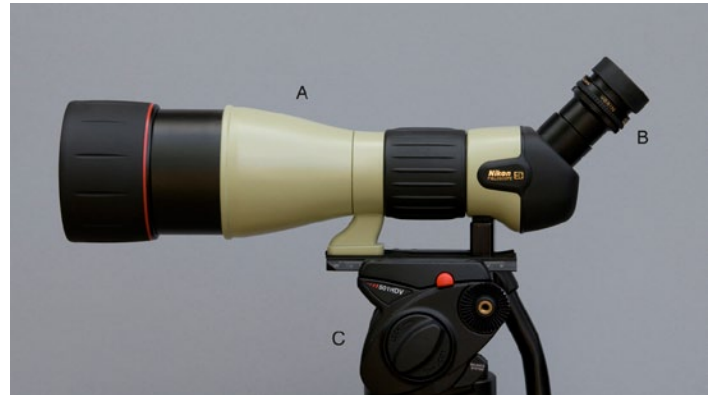
Figure 1. A) Nikon Fieldscope ED82-A, 1000mm focal length lens. B) 45° angled zoom MCII 25-75x removable (threaded) eyepiece. C) Manfrotto 501PLONG Rapid Connect Plate, mounted on Manfrotto 501HDV head, and Bogen/Manfrotto 3221W aluminum tripod.
