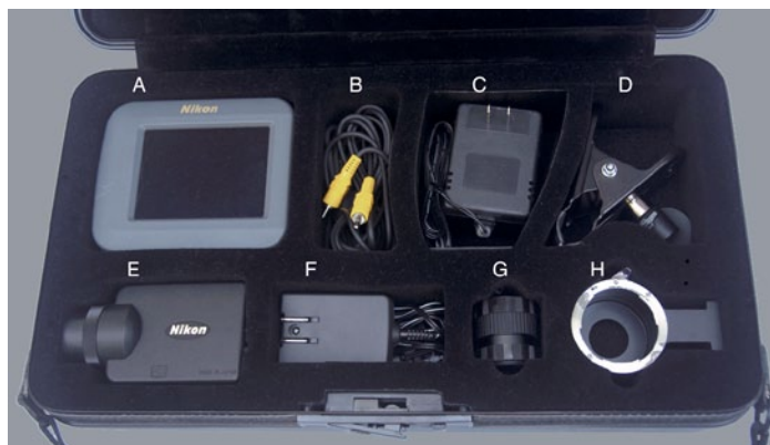
Figure 2. Nikon Field Image System MX: A) LCD monitor. B) RCA wire connectors. C) AC power adapter for monitor. D) Clamp to attach monitor to tripod leg. E) 80x CCD camera. F) AC adapter for camera. G) 12.9mm close-up lens. H) F-mount camera lens adapter.
