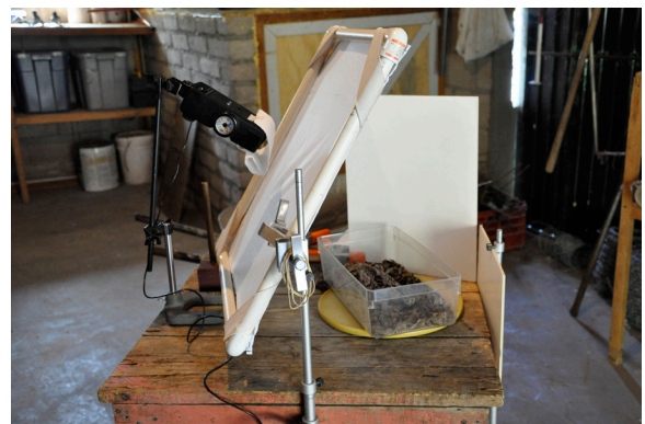
Figure 2. The lighting setup used most often consists of a single Vivitar 283 flash shooting through a 20"x24" diffusion panel of rip-stop nylon. This creates a single, large, diffused light source, which is positioned above and behind the subject. Foam board fill cards are arranged in front to reflect light back into the shadow areas. Rancho El Pinito, Sierra San Luis, Sonora Mexico. (The Cuenca Los Ojos Foundation).
